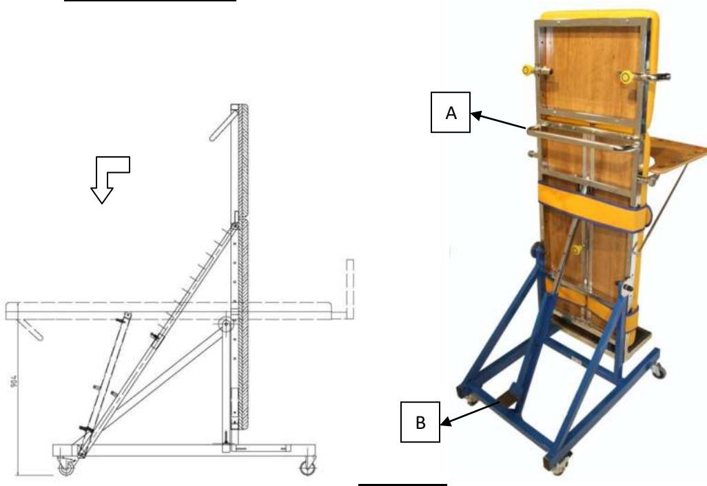
To swing the tilted table to the horizontal position, step on the pedal B and while assisting the movement pulling from the handle A towards the indicated arrow direction.
