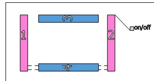
3.- Join the 2 cables from the block nº 4 with the ones from the block 1 and the same way connect the 2 cables from block 4 with the ones of the block nº 2.
